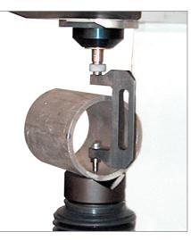
By applyng C shape indenter Art. 604, difficult points as: insides of tubes and near to hollows can be reached.
